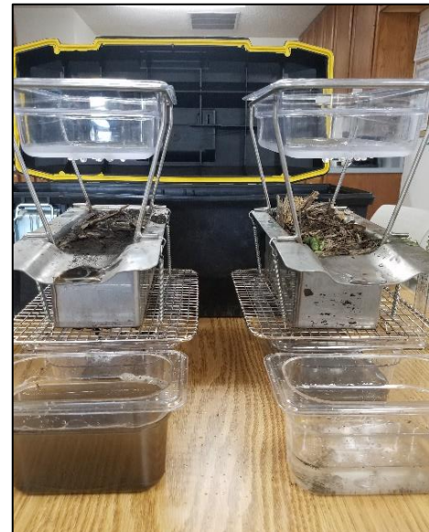
Rainfall simulator comparing conventional tillage (left) versus no-till with cover crops (right). Water runoff is collected in the front container.
